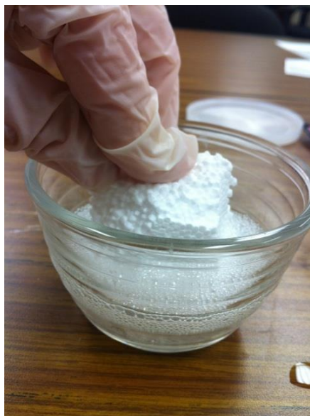
Fig. 5 Polystyrene dissolving in d-Limonene
