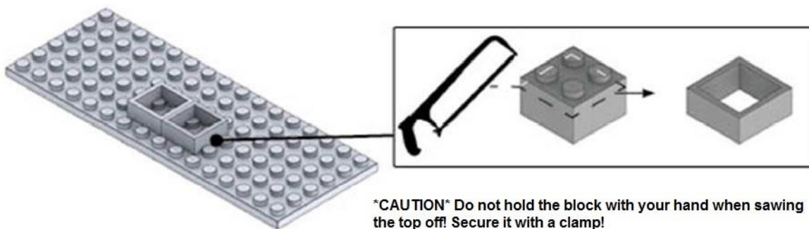
2x2 Lego blocks hold cuvettes well if their top is cut off
