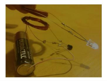
ADA Description: Battery powered transmission circuit with L.E.D. light to help demonstrate how wireless power transfer works. Caption: Wireless Electricity Transmission Circuit
