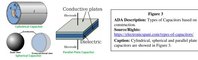
The value of the capacitor is determined by 3 physical factors: the amount of surface area of the parallel metallic plates (A); the separation or distance between the plates (d) and the insulating material or dielectric between the plates. The capacitance is given by the expression on Figure 4:
