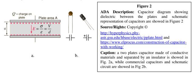
The capacitor stores electrons when there is a voltage applied across the plates. Even though the dielectric creates an open because it is an insulator, current flows in the conductors between the voltage source and the plates. This current, that appears to flow through the capacitor, is referred to as displaced current. Current can only flow
