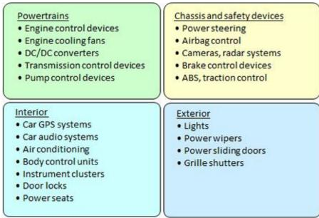
Table 1 Applications for aluminum electrolytic capacitors for automotive use[4]
