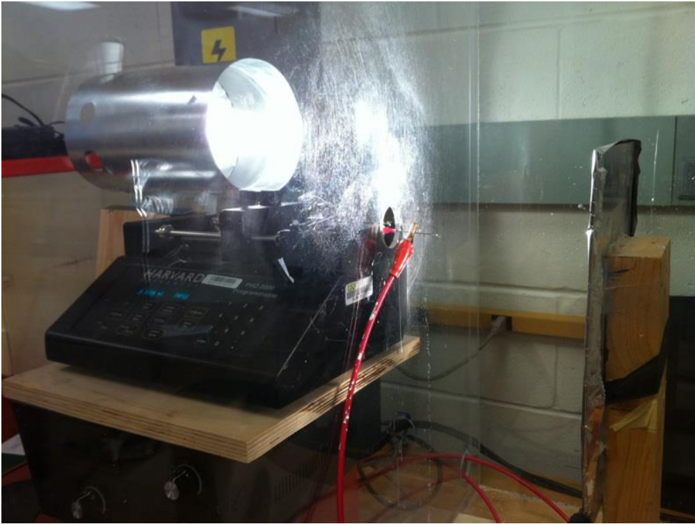
Fig. 4 Electrospinning equipment with fibers evident at the syringe tip.
