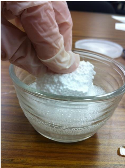
Fig. 5 Polystyrene dissolving in D'Limonene
