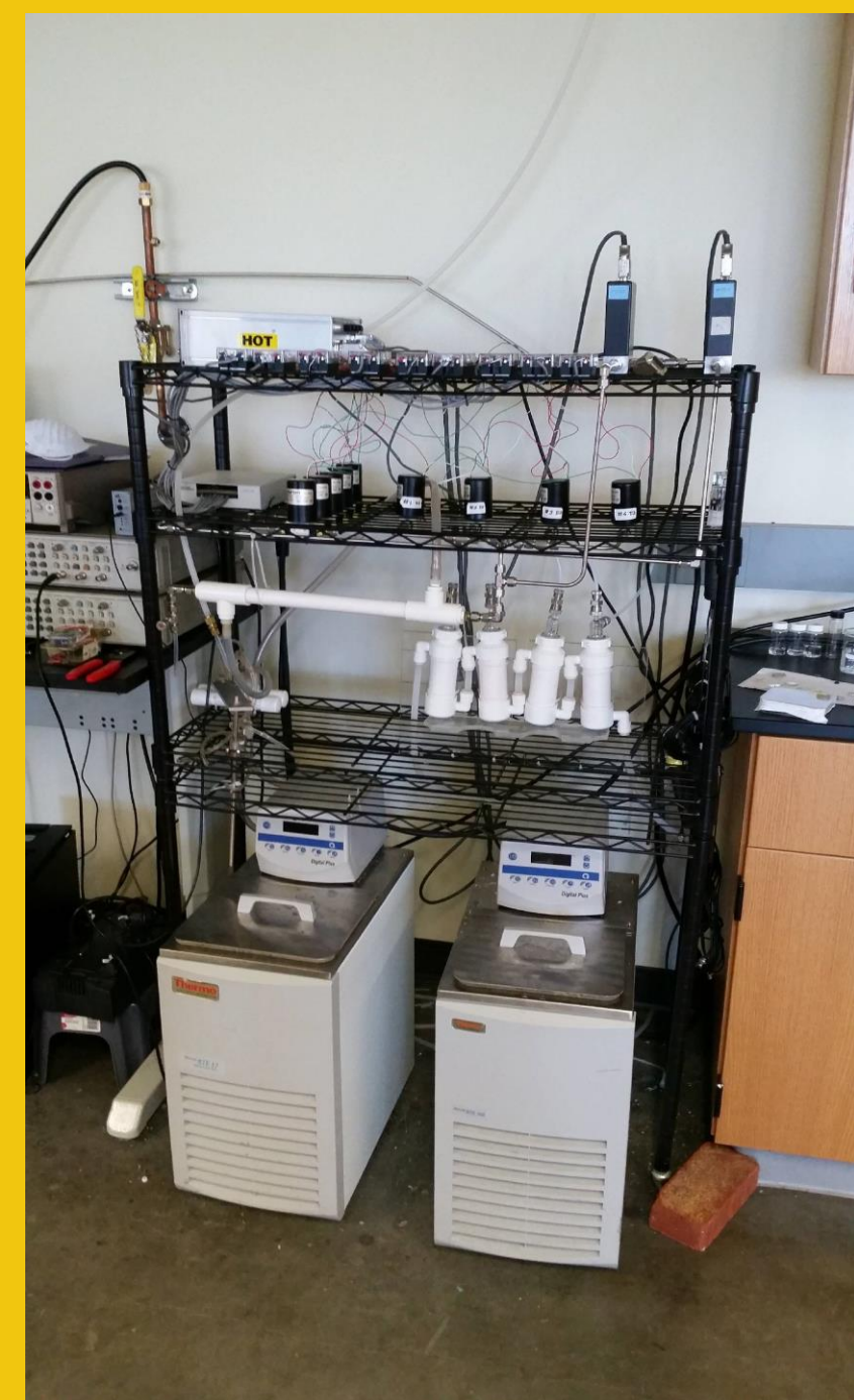
The full apparatus housing for organic vapors and polymer coated quartz crystal
