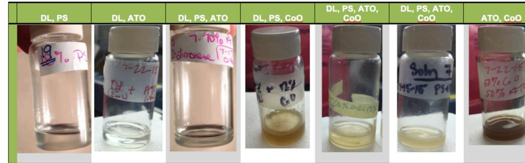
Figure 3: Mixed solutions of d-limonene, PS, ATO and CoO in glass vials after stirring with magnetic stir bar.
