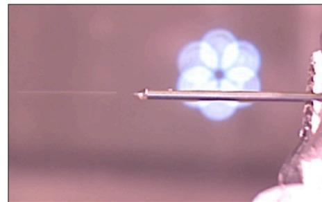
Figure 5: 150x magnification of the Taylor cone at the tip of needle with visible jet being released.
