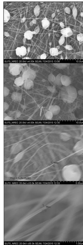
Figure 2: SEM pictures of nanofibers made of DL, PS, ATO and CoO.
