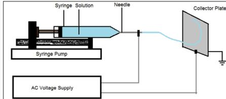
Figure 1: Illustration of the electrospinning equipment<sup>7</sup>
