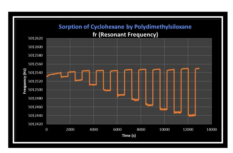
When equilibrium between the polymer and gas stream was reached, the additional frequency shift  $\Delta f$  was noted. The weight fraction ( $W_1$ ) of the organic species in the polymer film was calculated from
