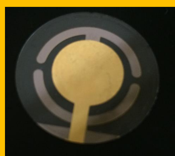
A 5mhz quartz crystal is coated with PIB
