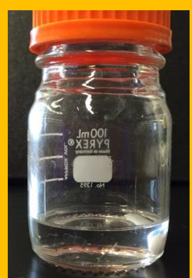
Coating solution of 15% polyisobutylene and chloroform
