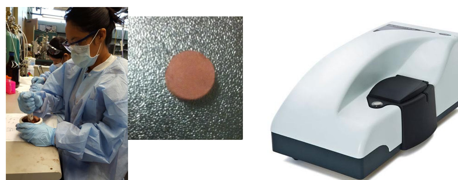
Fig. 2. Mixing powders with binding agent, pellet after sintering, Malvern particle size analyzer.
