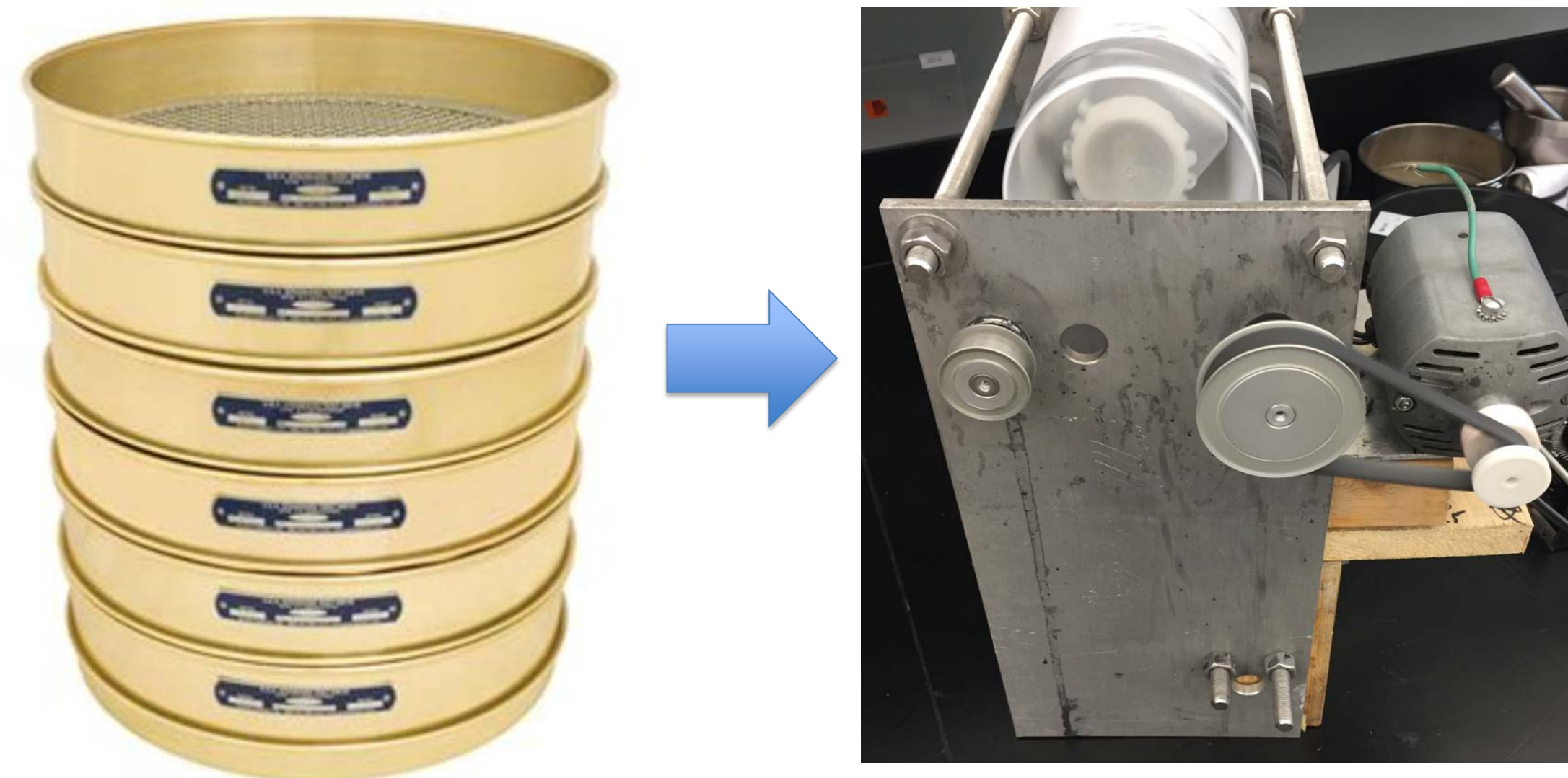
Fig. 2: Bimodal powder mixtures procedure using 316L stainless steel coarse powder.
