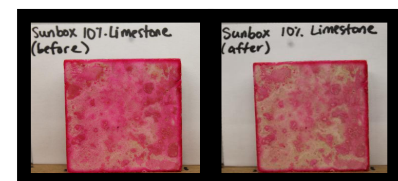
figure 2: Simulated Sunlight on Limestone
