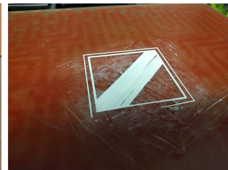
Fig 6. Failed Thin Sheet Print
