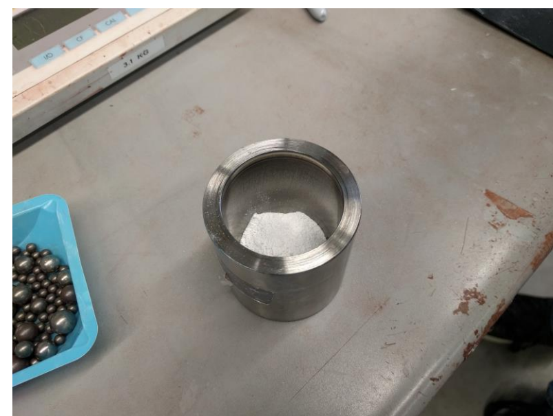
Fig 1. BST powder in container for ball milling
